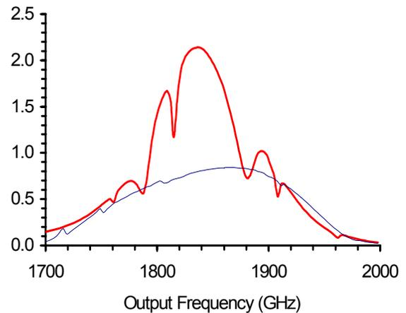
**Figure 2:** Calculated output power of the 1.9 THz balanced (dark) and unbalanced triplers. Input power of 2.5 mW is assumed.  $C_j(0)=1\text{fF}$  for the unbalanced tripler and  $C_j(0)=0.8\text{fF}$  for the balanced tripler.
