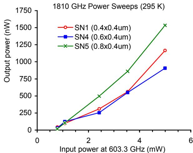
**Figure 5:** Output power measured at 1810GHz versus input power for three different multipliers at room temperature.
